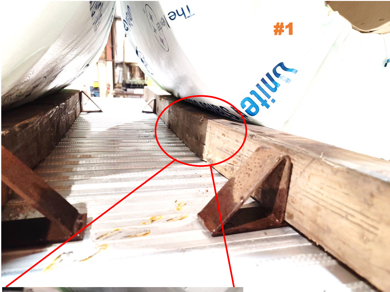
Image 1: Coil racks were not placed correctly under this coil.
