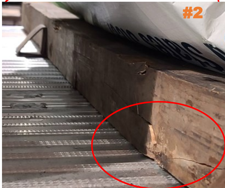
Image 2: Due to the coil racks being placed too far apart, the dunnage plank cracked. It may not seem like it but in the instance of a hard break this will allow enough movement for the coil to roll off of the trailer.
