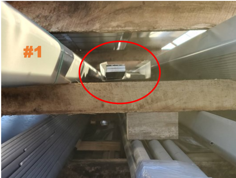
Image 1: A Grout Channel is placed in the middle of longer pieces of material on this load. There is no proper way to secure this item. As a result, the trailer will need to be taken back to the shipper plant to have the piece re-arranged on the trailer in order to properly secure.
