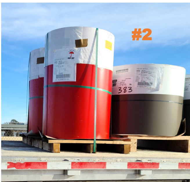
Image 2: Painted coils on skids should not be placed on the trailer side by side. These types of coils need to be placed in a single file line, going down the center of the trailer.
