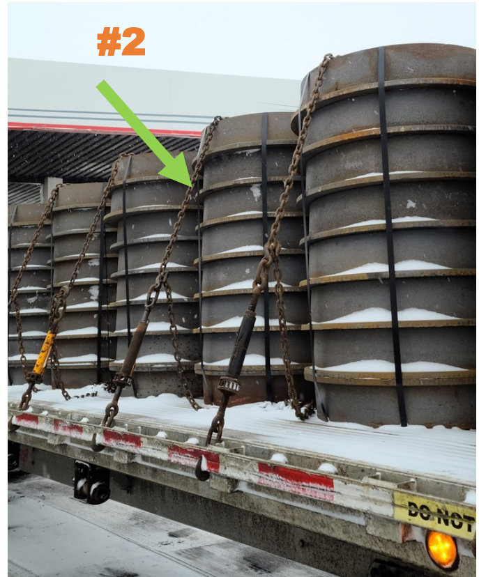
Image 2: Shows one way to secure center columns of manhole pieces by using chains.
