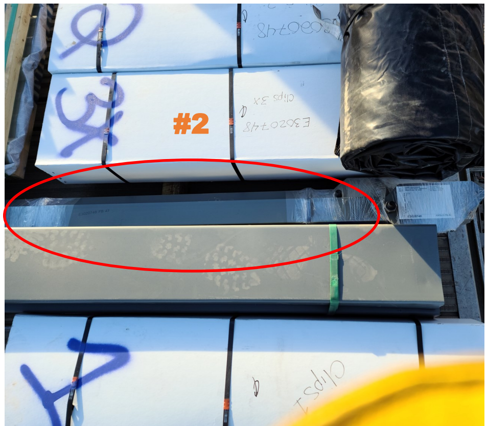
Image 2: A bundle of Angle Dew has been set between two boxes on this load. To properly secure this item on the trailer, the bundle of Angle Dew must be placed on top of the boxes or in another position on the trailer, to have direct contact with a chain or strap. Again, this would be another instance that the load would be rearranged by the shipper.
