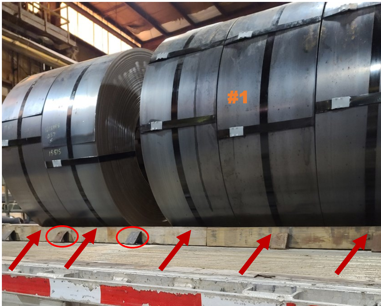
Image 1: displays another example of incorrect placement of coil racks. For these types of narrow coils, racks should be placed in the center of each coil, along with a dunnage plank.
